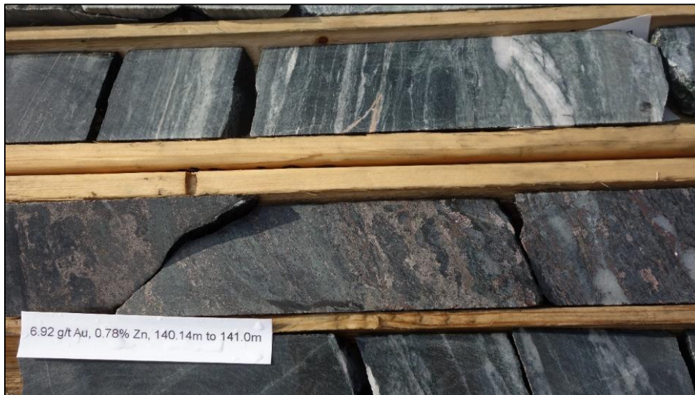
FIGURE 10.2 MINERALIZATION IN EM20-142 IN A DEFORMED AND ALTERED UNIT WITH BIOTITE AND GARNET PORPHYROCLASTS
