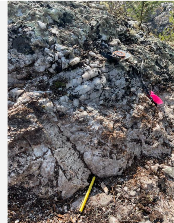
Coarse spodumene (lithium bearing pyroxene) in rock chip sample from Ruby Hill West pegmatite.
