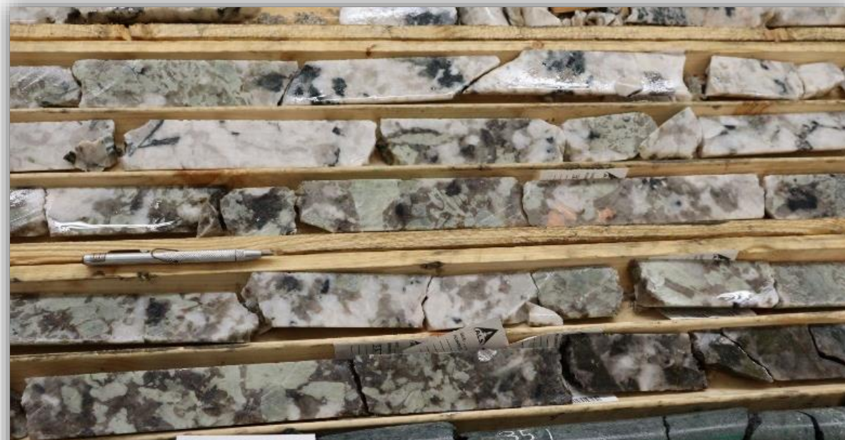
Spodumene rich part of RHW22-006 intercept, this part is from the 3.7m at 2.70% Li 2 O
