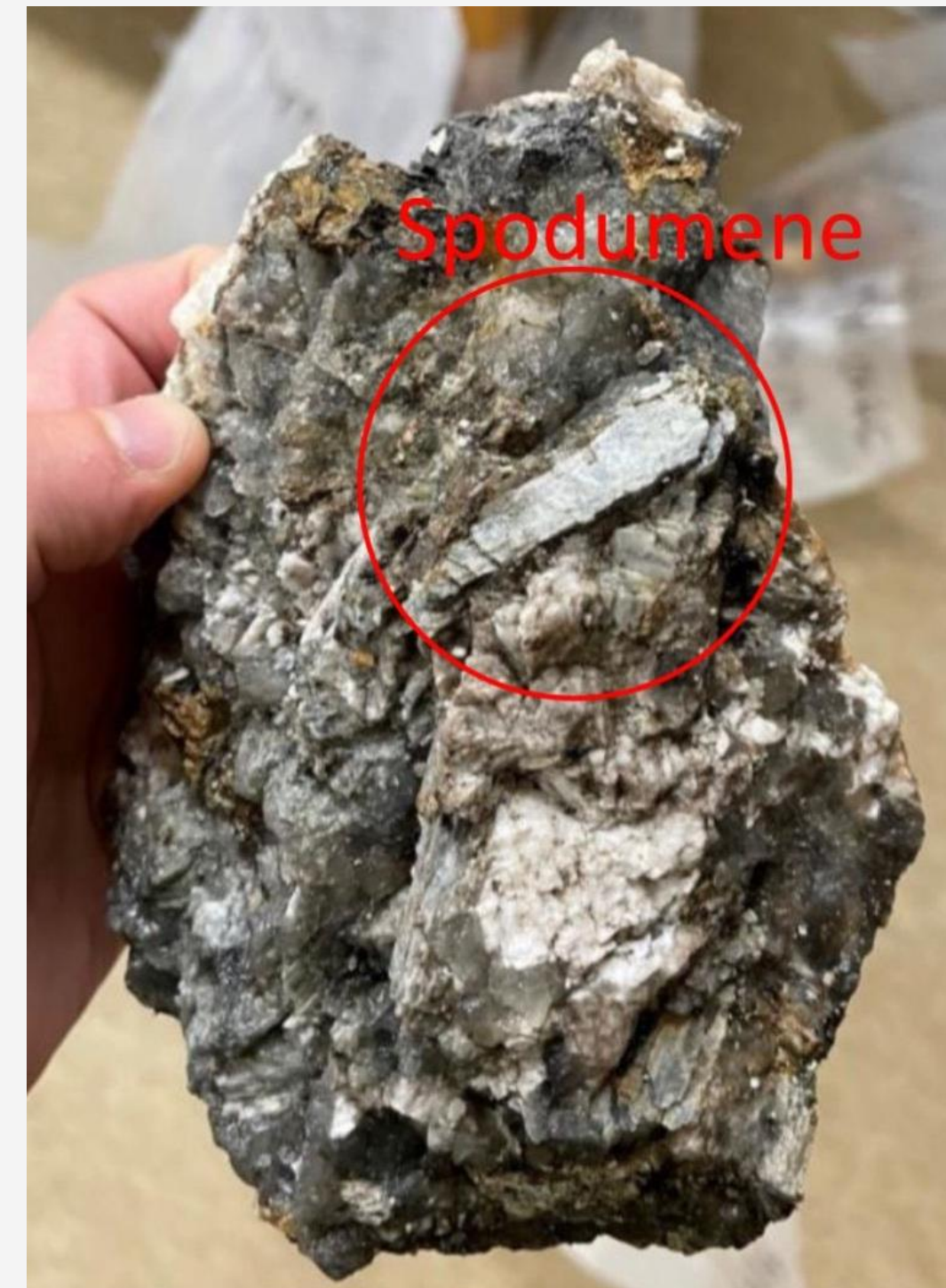
Coarse spodumene (lithium bearing pyroxene) in rock chip sample from Ruby Hill West pegmatite.
