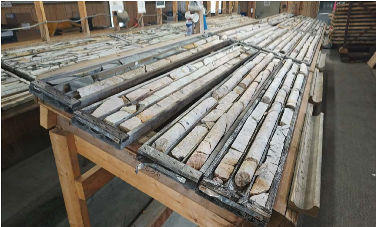
Figure 6: RHW-08-003 core displaying pegmatite (80m of cumulative length).
