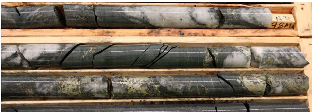
Figure 3: Drillhole EM22-272, Chalcopyrite associated with quartz veins between 76.65m and 81.4m.
