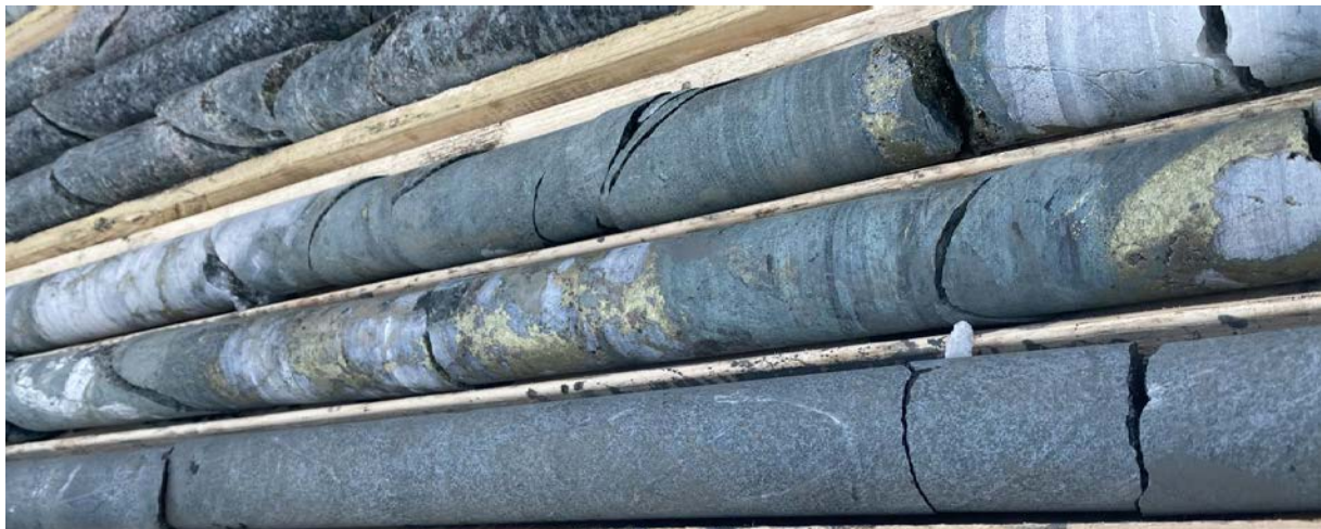
Figure 1: Chalcopyrite mineralisation in core from drillhole EM22-272 - Michel prospect
