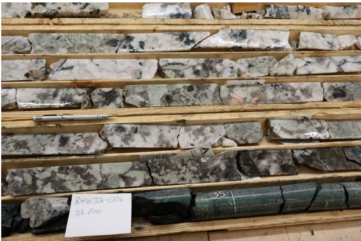
Figure 3: Spodumene pegmatite, RHW22-006, half core. The other half will be sent to ALS laboratories for assays on 28/04/2022
