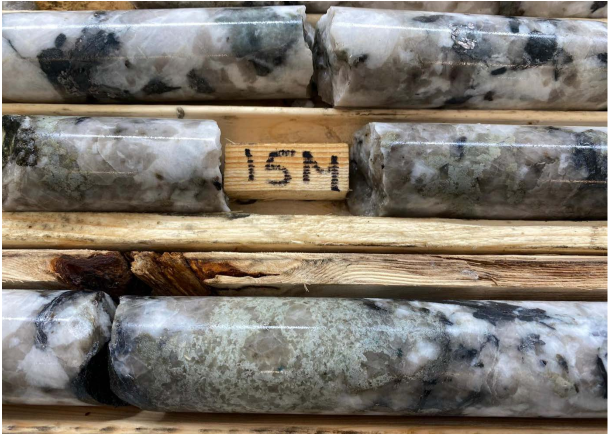
Figure 9: RHW22-006 pegmatite close-up, the black mica is masutomilite (Rb rich mineral), with quartz and feldspar visible
