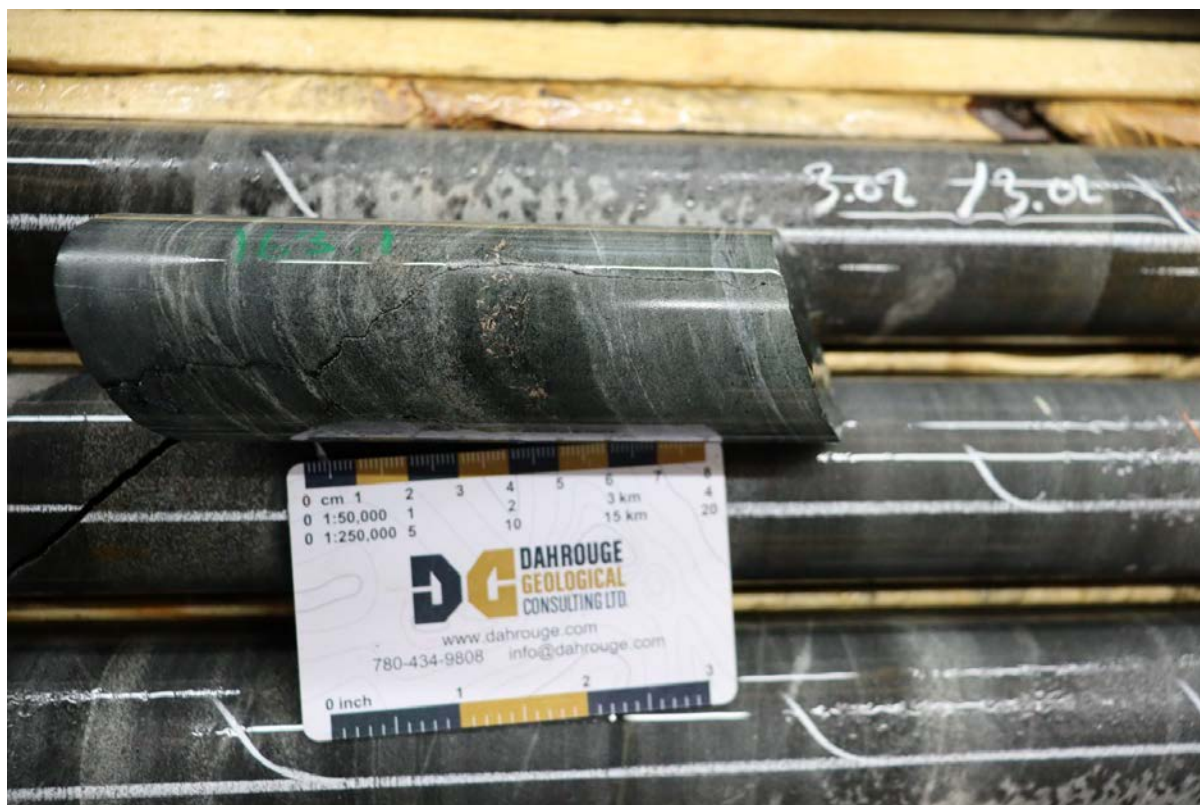
Figure 10: Nickeline in a small vein within a deformed ultramafic intersected in hole RHW22-003.
