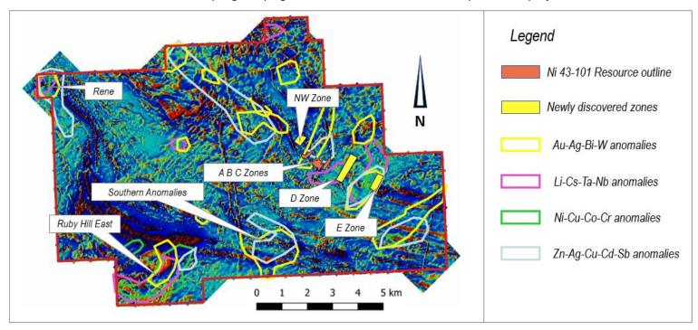
Figure 1: Soils anomalies over 1st derivative magnetic image
