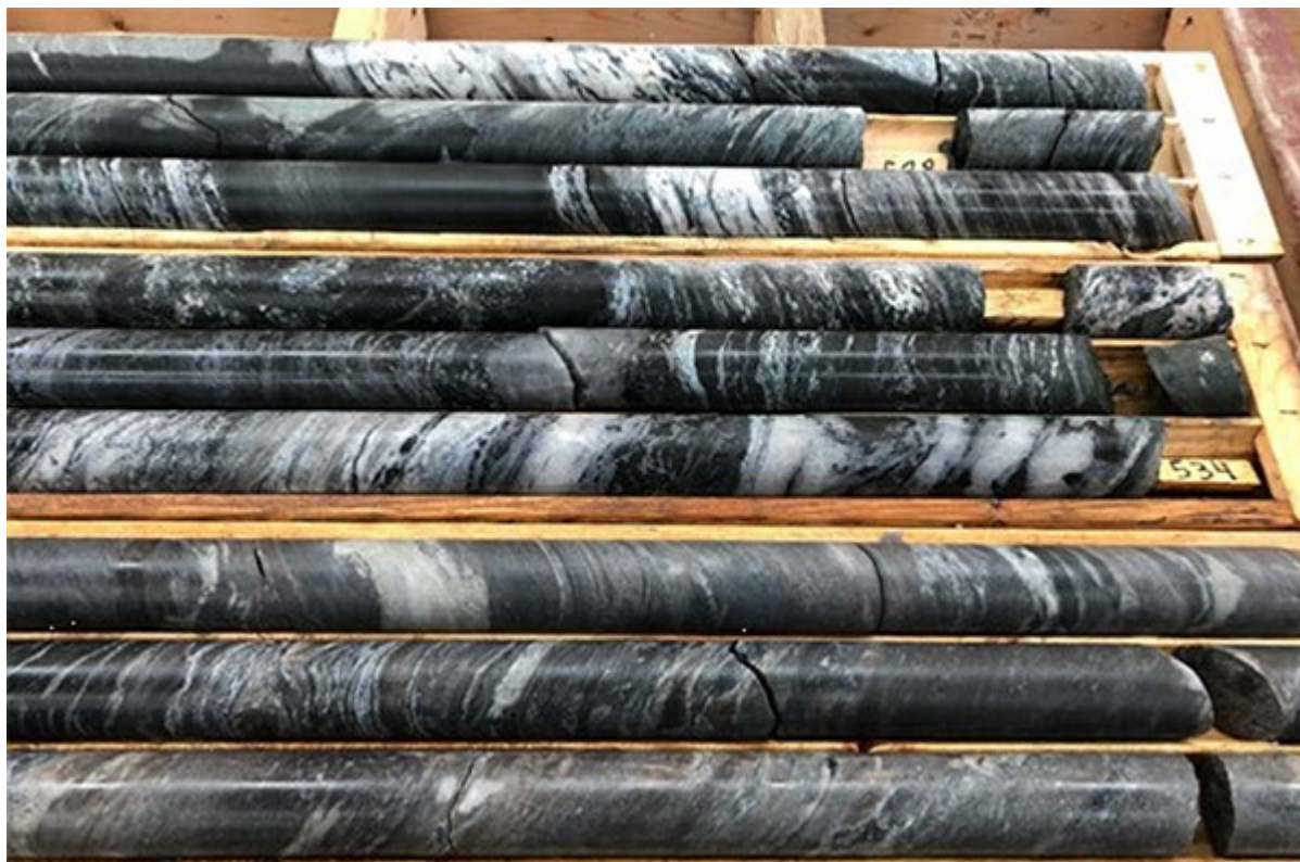
Figure 4: Quartz and quartz-tourmaline- carbonate veining with stringers and disseminated sulfides (core diameter 47.6mm) in biotite and sericite altered rock
