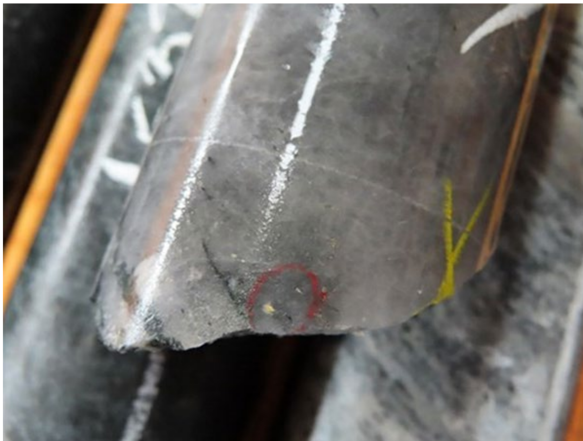
Figure 5: Visible gold grain in quartz-tourmaline vein, hole EM20-132, ~532.7m (core diameter 47.6mm)
