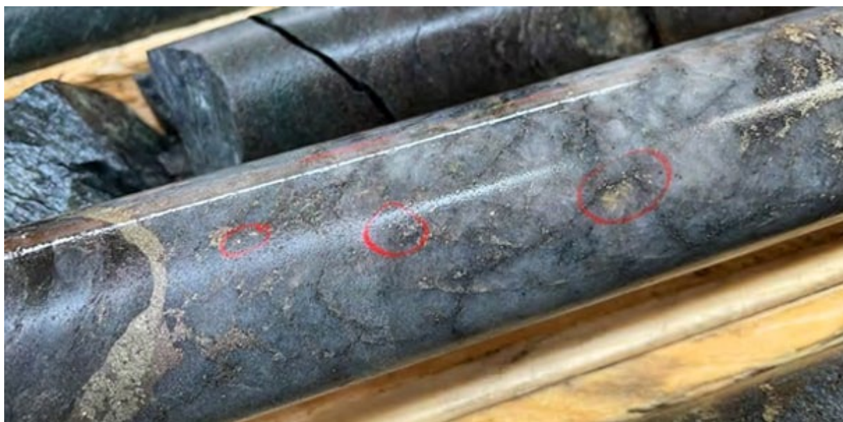
Figure 4: Visible gold in quartz-pyrrhotite-pyrite-sphalerite veins EM21-146 – NW Zone (for reference, core diameter 47.3mm)
