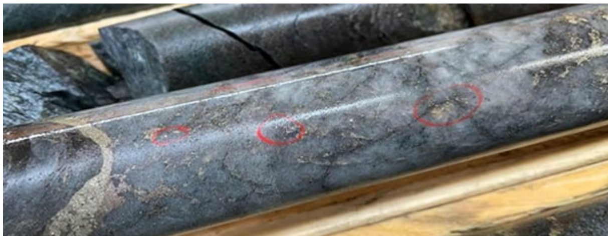
Figure 1. Visible gold circled in red from a core drilled at NW Zone (hole EM21-146) 600m NW of the existing resource
