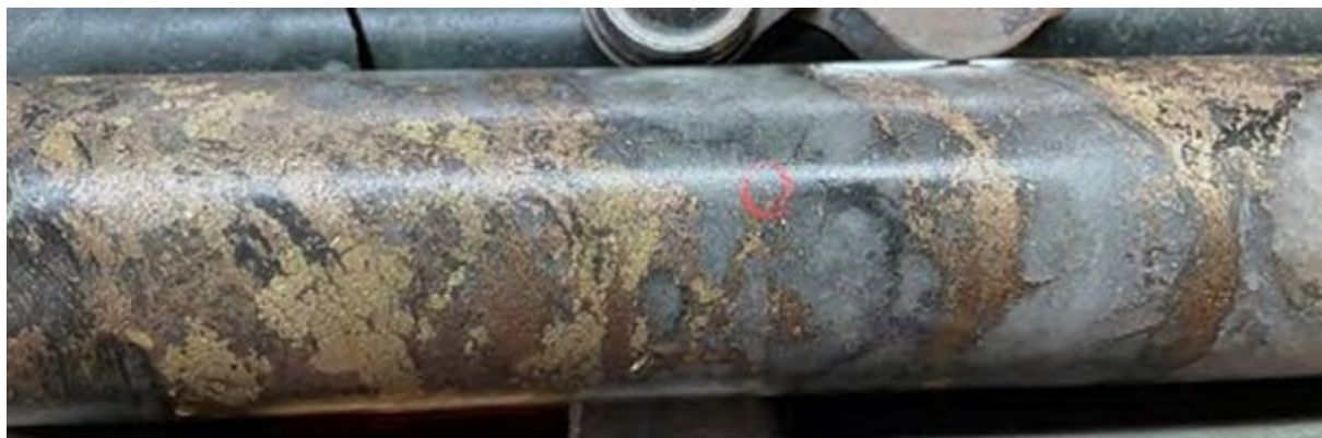
Figure 5: Visible gold in Quartz carbonate pyrrhotite pyrite sphalerite vein EM21-146 – NW Zone (for reference, core diameter 47.3mm)
